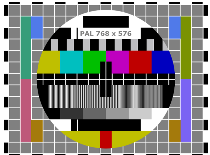
Figure 6: Output frame from the hardware simulation example (Scale-down of 768x576 to 640x480)
