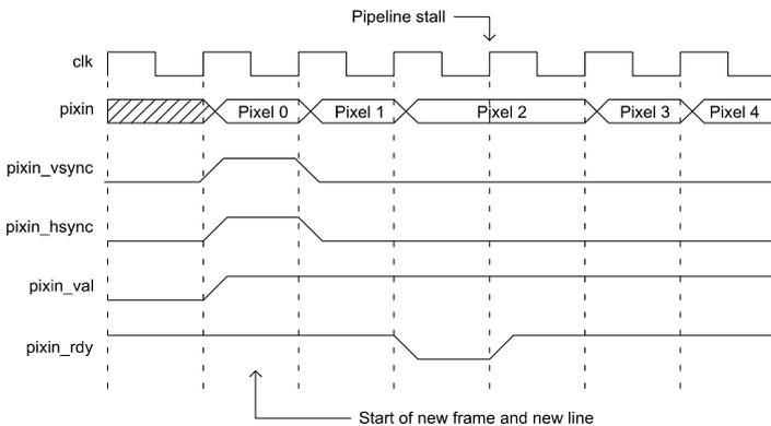
Figure 4: First line of a new frame
