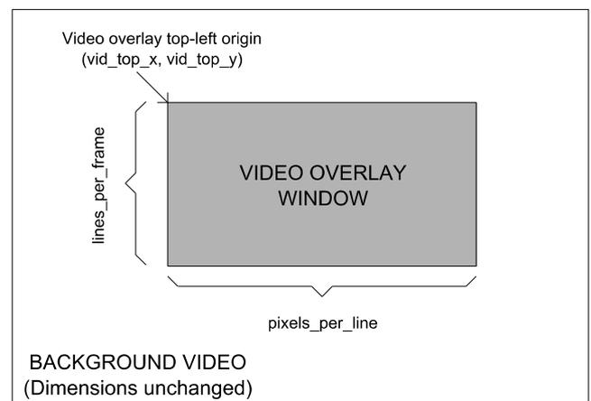
Figure 2: Video overlay window positioning and size
