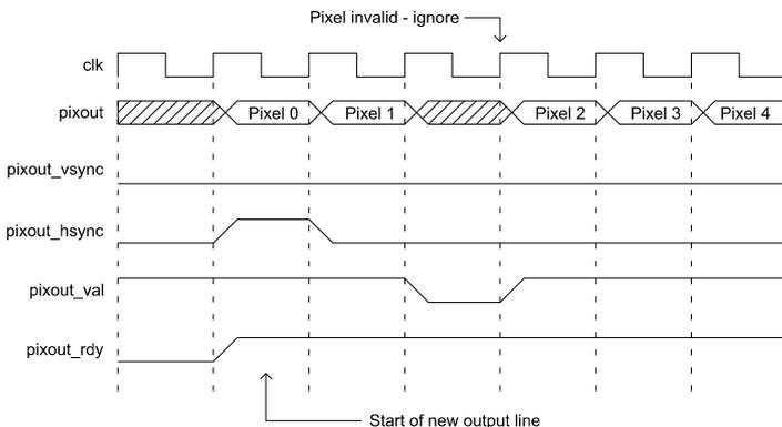
Figure 5: Video overlay output showing invalid pixel
