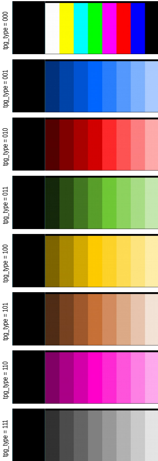
Figure 2: Different test pattern types. An SMPTE 296M (720p) output video stream is shown as an example
