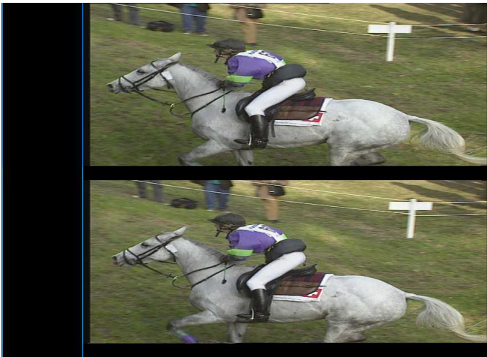
Figure 4: Output image from the simulation showing the separate fields in the BT.656 encoded video
