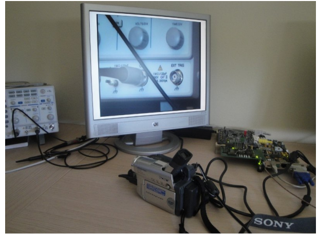
Figure 9: Photo of the deinterlacer test setup
