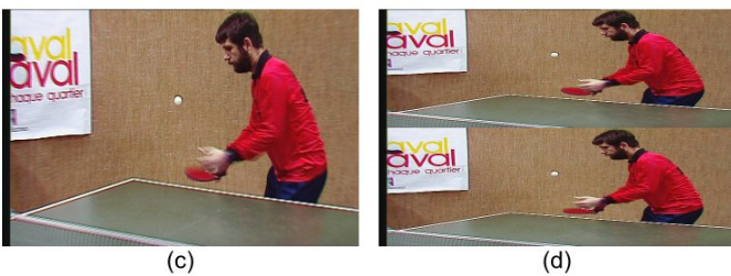
Figure 4a & 4b: Results of decoding a full PAL interlaced frame into its constituent fields. Figure 4c & 4d: Results of decoding a full NTSC interlaced frame into its constituent fields.
