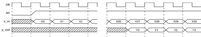
Figure 2: FIR filter input/output samples
